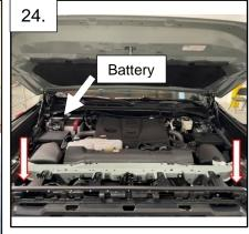
25. Locate one light connector lead of the main harness and route it down behind the passenger headlight and across the inner bumper to the driver side to the backside of the vent. With some **patience**, attach two splitters to create one connection between the three lights. Reach into the inner fender and connect to the main harness. Repeat for the passenger side taking care to make sure each harness is connected. (Image with grill removed for clarity.)
