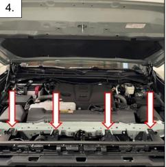
5. Disconnect the electrical connectors on the top of the grill near the top of the radiator (arrowed). For TRD models, there are two on the driver side and two on the passenger side. For non-TRD models, there are two on the passenger side and one on the driver side.
